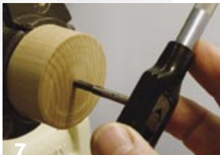
7 Drill and tap the wasteblock. Secure an #8-32 screw from the backside with CA glue.
