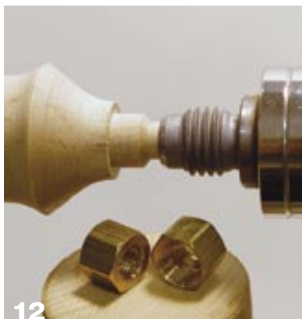
12 Check the diameter of each compression nut, then cut the tenon to fit the interior.
